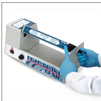
4. Depress and hold the Release button, slide Lock Shaft into Platform through the housing. Hand-tighten Lock Shaft fully into place then let go of the Release button
