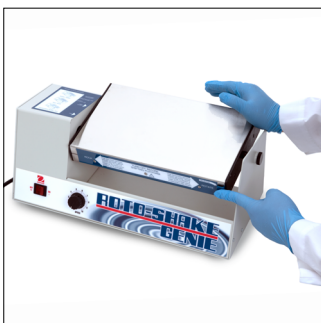
5. For rocking, press Release button, align Pin Slot on Platform with Pin on housing and shift Platform to the left, then let go of the Release button
