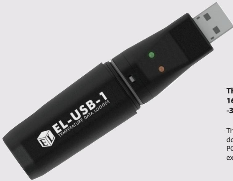
The EL-USB-1 data logger measures and stores up to 16,382 temperature readings from a temperature of -35°C to +80°C.
