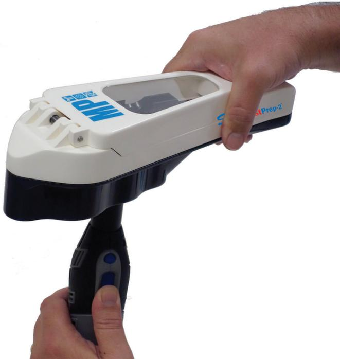
The angular position of the rotary tool relative to the *Super FastPrep-2* may be adjusted by removing the 3 screws at the base of the *Super FastPrep-2*, rotating the adapter to the desired position, and then replacing the 3 screws. See the picture below.
